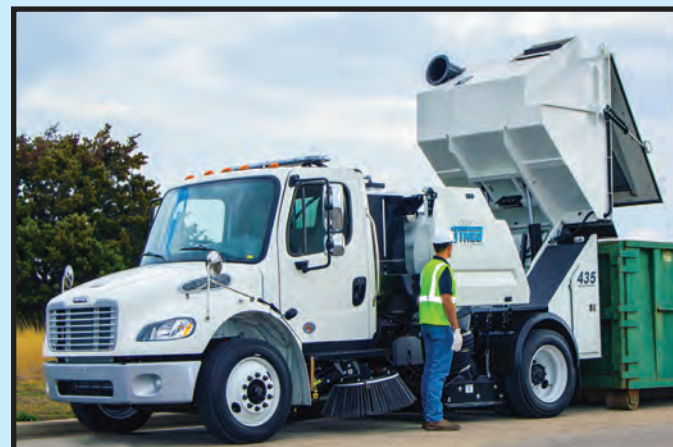
Dumping into a 30 yard Container
