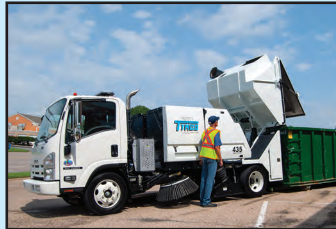
Dumping into a Low-Profile 30 yard Container
