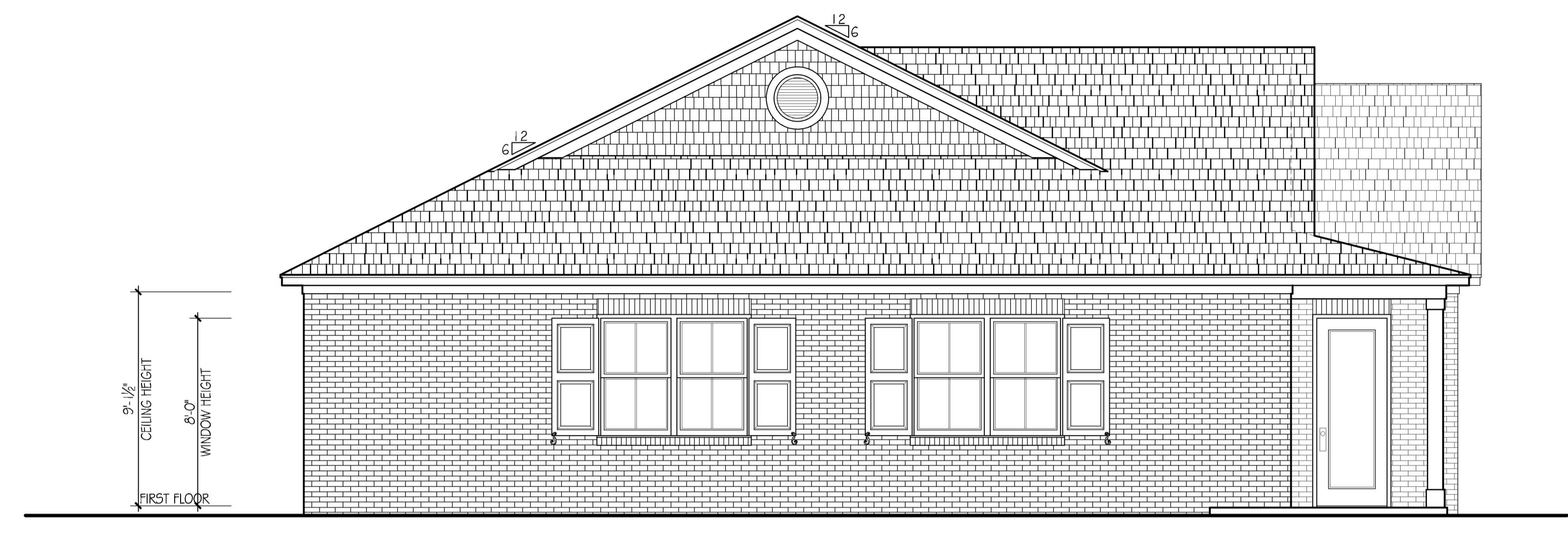
UNIT 'A' BUILDING #2 - FRONT ELEVATION SCALE: 1/4"=1'-0"
